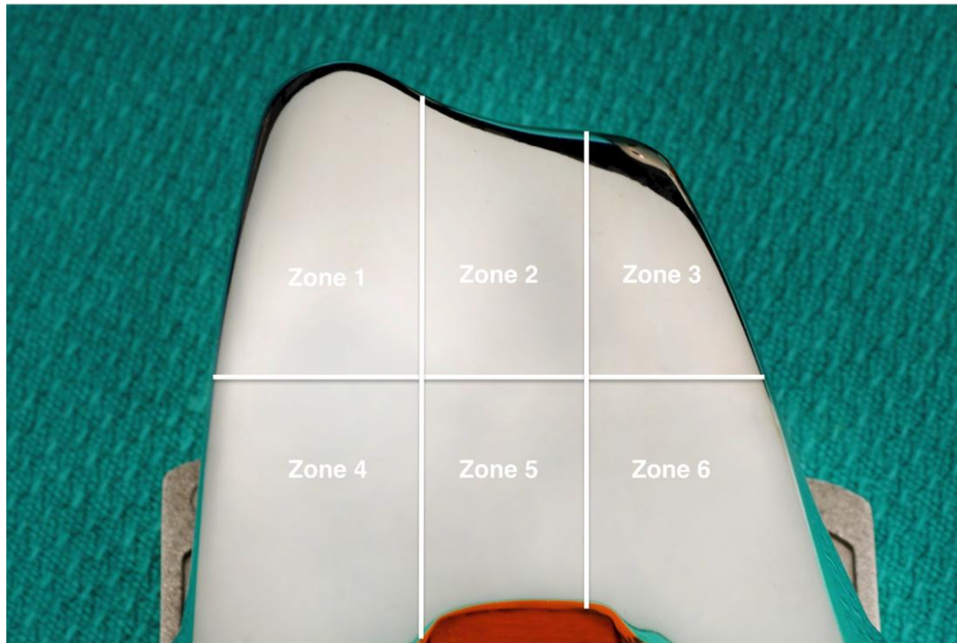
Figure 5-2. The trochlea of each femoral component was divided into 6 zones in a consistent pattern. (Photograph taken at the LHSC Implant Retrieval Laboratory)
